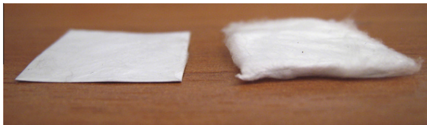
Fig. 2. The gross view of electrospun mats fabricated via conventional (left) or light emission array electrospinning (right).
